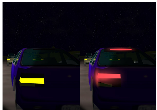
Fig. 3. Alternative lighting: tail lamp on, brake lamp on.
